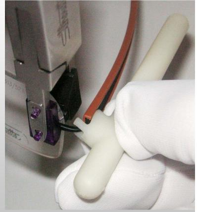
Hold the lens fixation by hand (fullrim or nylor) or with mounting pliers (rimless frames). Close the temple by approx 30°. Place inclination lever on side part and hinge and adjust inclination angle as required.
